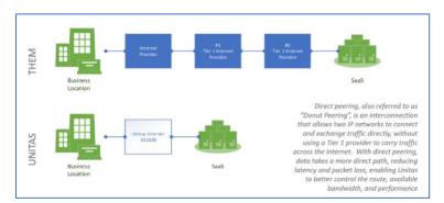
The Unitas difference is that we built our IP network to bypasses the Tier 1 core entirely, wherever possible, and take customer traffic directly to its destination, traversing the fewest number of networks and interconnections. Direct peering is an interconnection that allows two networks to connect and exchange
